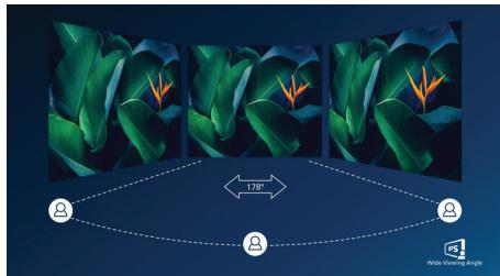
IPS displays use an advanced technology which gives you extra wide viewing angles of 178/178 degree, making it possible to view the display from almost any angle - even in 90 degree Pivot mode! Unlike standard TN panels, IPS displays gives you remarkably crisp images with vivid colors, making it ideal not only for Photos,
