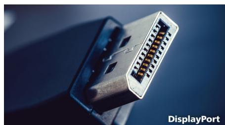
With DisplayPort-out you can connect multiple high resolution displays with just one cable from your first display to the PC. The ability to daisy chain multiple displays enables
